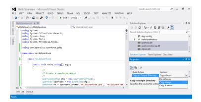
Figure 15: .Net compilation - copy to output
